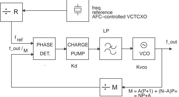
LO–signal is generated by SHF VCO module. VCO has double frequency in GSM1900 and x 4 frequency in EGSM compared to actual RF channel frequency. LO signal is divided by two or four in HAGAR (depending on system mode).
